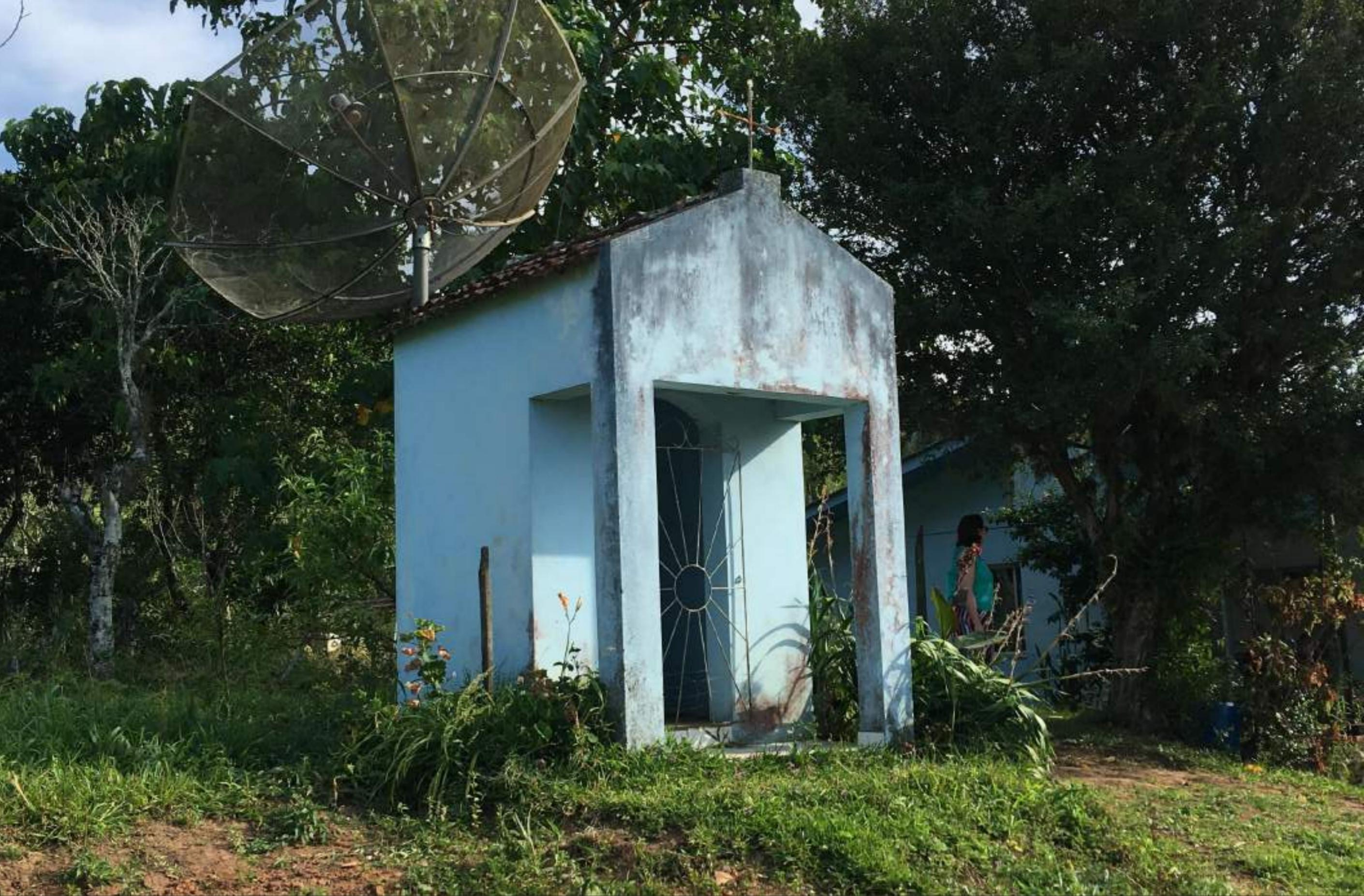
The building is located in the countryside, on the edge of a privately owned path, accessed by a dirt road, on slightly hilly terrain. Rectangular floor plan accessed by an iron leaf gate, lintel of the opening in full arch. No windows. Cover two waters with ceramic tiles. Wooden plywood lining and wooden lining wheel. With a smooth pediment, topped by an iron cross and supported by two smooth pillars. Ceramic floor.
